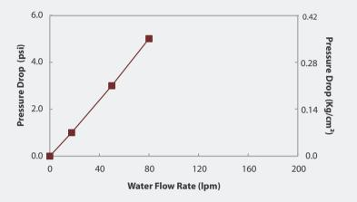
1 μm *ClariSure*®*P*L, 10" Standard Cartridge Filters
