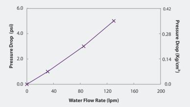
2.5µm ClariSure®PL, 10" Standard Cartridge Filters
